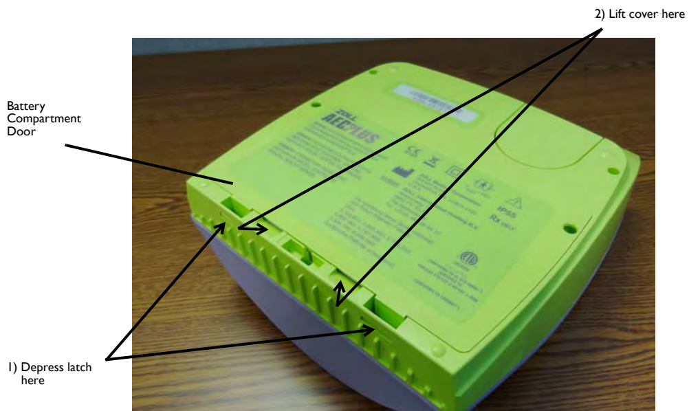
Figure 7: Removing the Battery Compartment Door
