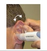
Pull tab to remove the ear tip from the handle and dispose of properly.
