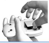
With the meter powered off, turn it over. Press the latch gently inward and lift the cover. Remove the old batteries, if necessary.
