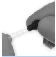
Firmly insert the end of the capillary tube into the capillary bulb. Completely insert the tube into the bulb to break the bulb diaphragm.
