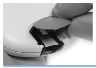
With the meter powered off, use your thumbnail to open the cover of the test strip guide by pressing its front edge upward. Move the cover safely away from the meter. Then rinse the cover with water or wipe it clean.
