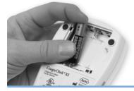
Position the batteries according to the diagram inside the battery compartment. Replace the cover. Turn the meter back over.
