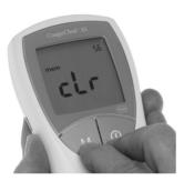
With the meter powered off, press **and hold down** the M button **M**. While you are holding down the M button, press the ON-OFF button **and then hold down both** buttons for at least 5 seconds.
