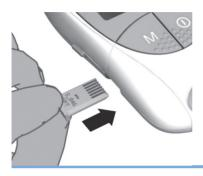
Make sure the meter is powered off. With the code number facing up, insert the code chip into the code chip slot until it snaps into place.
