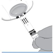
Slide the test strip into the test strip guide in the direction of the arrows until it stops.
