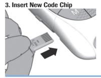
Slide the new code chip into the code chip slot until it snaps into place.
