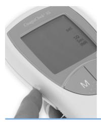
Note: When you go to Setup mode, the date format, date, time format, and time settings appear first. Press the SET button is to move past the date and time settings to get to the advanced settings.
