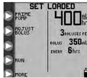
Figure 7C. Opening menu for Intermittent Feed mode with a Feed-Only set.
