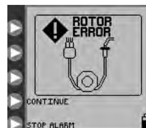
Figure 26. Rotor Error screen. Re-load the set tubing and press CONTINUE .
